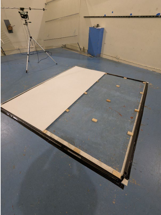
Figure 3 – Specimen partially installed over spacers
